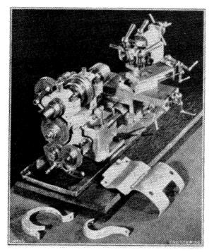
The threads were turned off a phosphor-bronze screw to leave a piece of stock out of which the main bearings had to be made, and its size governed the diameter of the mandrel. The mandrel was machined from a piece of a truck axle, and although it had been annealed it was a difficult job for the only high-speed steel lathe tool the workshop possessed. The leadscrew and a brass nut were made on a Sunday, and, with a rack and pinion from a damaged typewriter, were hidden until required.
